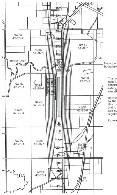
This map shows the maximum height of obstructions consistent with aviation safety, measured from the elevation of the runway.
